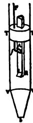
FIG. 2.—Organ pipe fitted with beating reed. AL, Beating reed. R, Reed box. F, Tuning wire. TV, Feed pipe. VV, Conical foot. S, Hole through which compressed air is fed.
